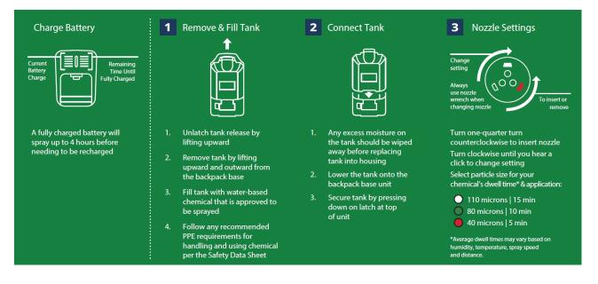
Please refer to the Backpack Sprayer Quick Start Guide for more detail IMPORTANT: It is recommended to use only the red 40micron nozzle setting for Callington disinfectants.
